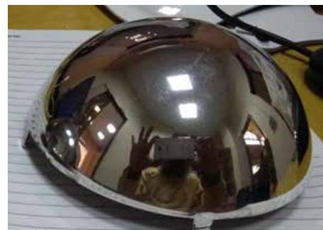
Figure 4. Aluminium layer by PVD process on Powder Coated base
