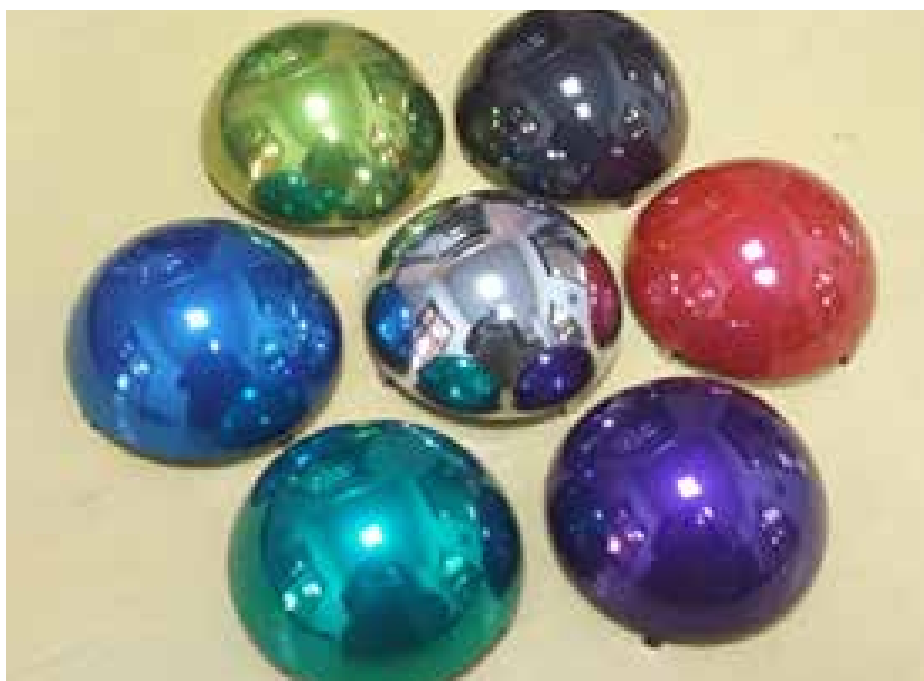
Figure 2. Nano Coating of Silver on PU base by Spray Metallization Process
