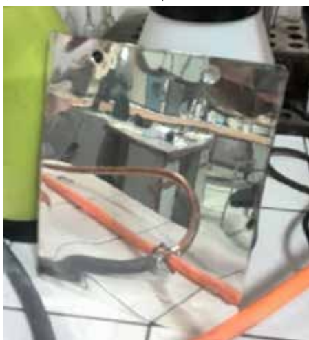
Figure 2. Nano Coating of Silver on PU base by Spray Metallization Process
