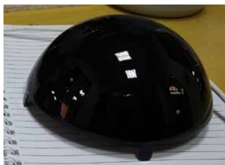
Figure 3. Base coat of Epoxy-Polyester Hybrid Powder Coating
